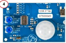
To adjust the length of time the relay is active, use the potentiometer, R7. Turn it counter-clockwise to increase the relay-on time and vice versa. Relay on is indicated by the LED, D2.
