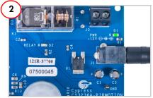
The CY3236A-PIRMOTION board is preprogrammed with firmware designed for the CY8C27443 PSoC device. Power the board using the 12-V adapter at the power jack, J1.Esure that the shunt is not placed on J4.
